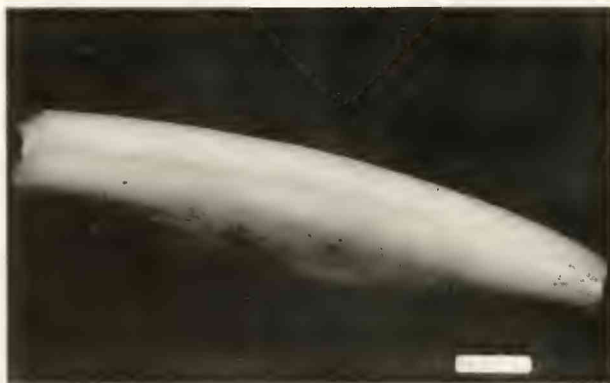
Fig. 12: Rodent incisor (Guinea Pig) subjected to a vertical load parallel to the anterior part of the tooth (gnawing load) with the help of Universal Testing Machine (UTM). The vertical cracks were observed confirming the presence of the stresses as observed in FEA analysis (scale bar = 1 mm).
