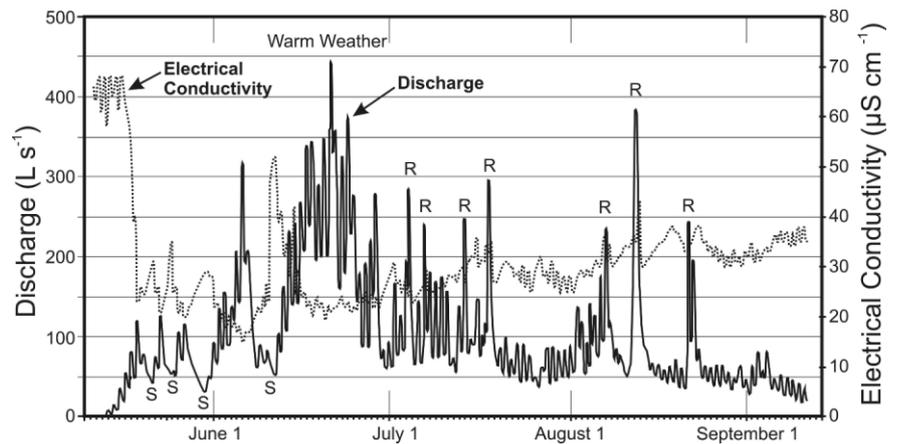
**FIGURE 5:** Hydrograph of the melt water stream at Reichenkar rock glacier (solid line) and electrical conductivity (stippled line) for the period from mid May to mid September 2002. Major snowfall events (S) with reduced discharge and rainfall events with peak discharge (R) are indicated.
