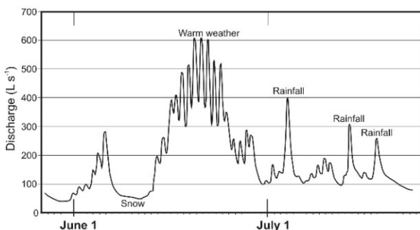
**FIGURE 7:** Hydrograph of the melt water stream at Kaiserberg rock glacier for the period May 27 to July 24, 2002. Peak discharge in June was caused by a period of dry and warm weather. The peaks in July were caused by rainfall events.
