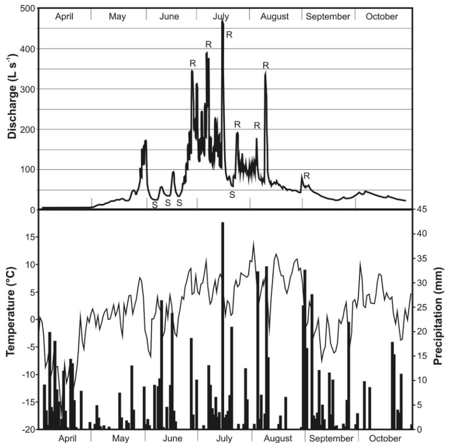
**FIGURE 6:** Hydrograph of the melt water stream emerging from the Kaiserberg rock glacier for the period April to October 2001. Snowfall events (S) and peakfloods caused by rainfall events (R) are highlighted.
