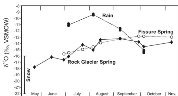
**FIGURE 8:** Oxygen isotope composition of the rock glacier spring, fissure spring, as well as of rain and snow at Reichenkar rock glacier during the period from June to November 2001. The snow profile was sampled in April.
