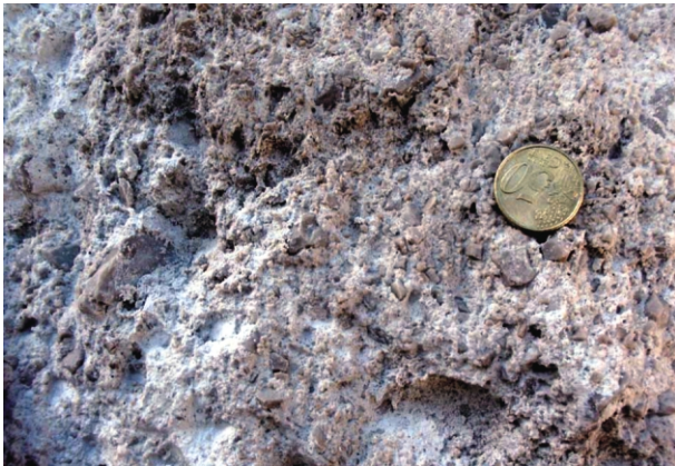
FIGURE 4: Compact limestone material of the sturzstrom deposits. See fig. 5 for grain size distribution.
