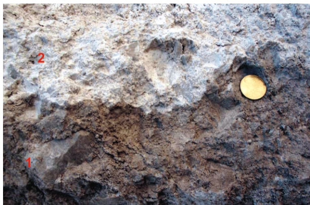
FIGURE 8: Sharp boundary between crushed and highly compacted dolomite (1) and limestone (2) material.
