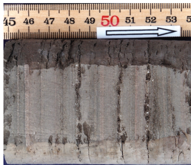
FIGURE 4: Depth 840m. Thin layered banded clay mainly reworked "Haselgebirgston" (grey, greenish, reddish). The variety of colours and grain-size of the thin layers are due to different sources ("Haselgebirge" and "Werfener Schichten"). Some of the layers show graded bedding (e. g. 46 cm on the scale). Arrows on the scale point to the top.
