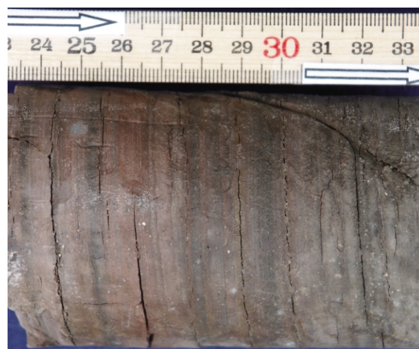
FIGURE 5: Depth 820m. Grey and reddish reworked "Haselgebirgston". Fissures on the surface of the core paralleling the bedding are perhaps caused by different clay content due to desiccation. Arrows on the scale point to the top.
