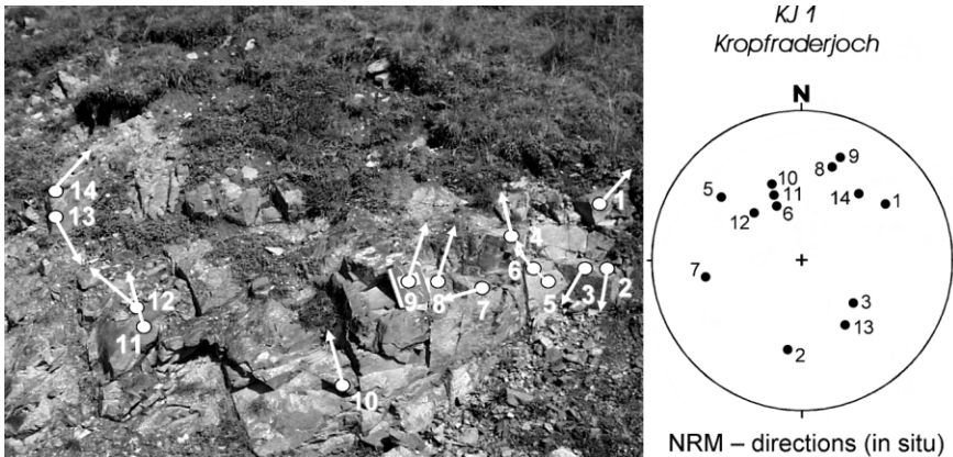
FIGURE 9: Directions of the natural remanent magnetization (NRM) at the Kropfrader Joch.
