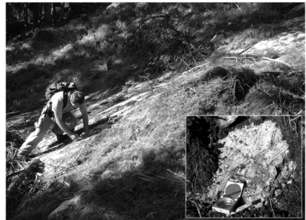
FIGURE 6: In-situ orthogneiss with gently E-dipping (mean azimuth/dip: 100/30), polished major sliding plane of the Köfels rockslide (between Köfels and Schartle, at approx. 1800 m a.s.l.).
