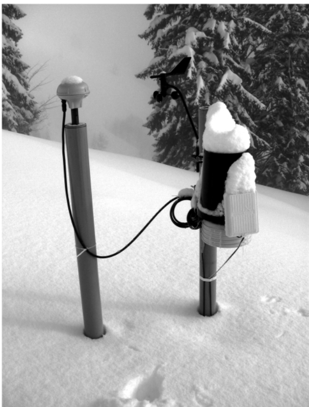
FIGURE 12: Winter impressions at Aggenalm test site. Main sensor node with GNSS sensor (Novatel Smart V1G-Antenna) and weather station.
