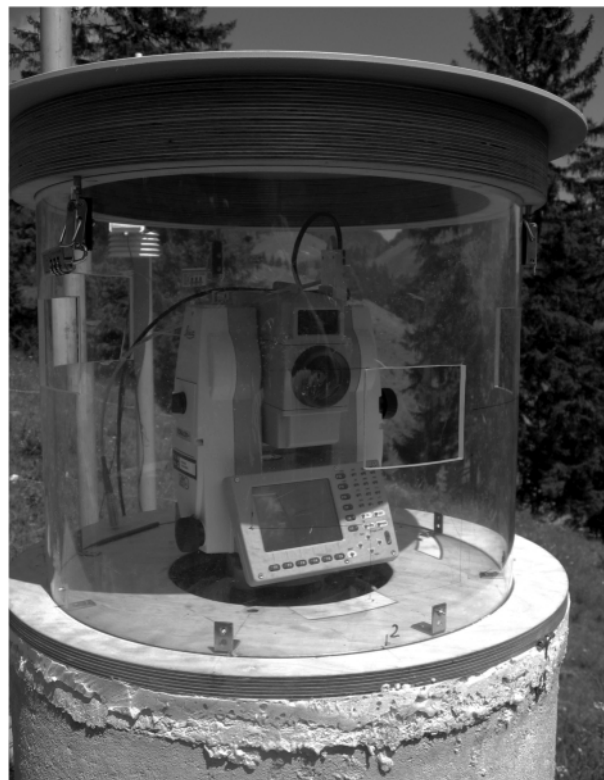
FIGURE 6: The IATS prototype in its housing at the Aggenalm landslide test site.
