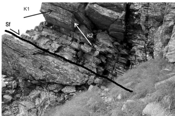
FIGURE 7: Foliation (Sf, black line) in the upper part of the mass movement, dipping downslope, enabling in combination with two orthogonal vertical joint sets (K1 and K2) sliding on cleavage planes; Picture taken from behind the ridge.
