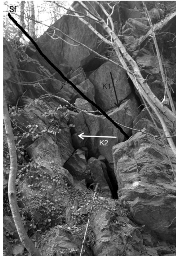
FIGURE 8: Foliation (Sf, black line) in the lower part of the mass movement, dipping into the slope, enabling spreading between cleavage planes due to gravitation/tension forces at the steep slope; in combination with orthogonal joint pattern (K1 and K2) creeping movement is eased.
