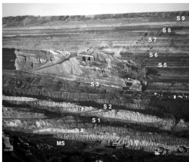
FIGURE 4: Overview of the highwall at the centre of mine Schöningen Südfeld showing the entire Paleogene section as exposed in fall 2007 (MS – Main Seam, S1 to S9 – Seam 1 to Seam 9 according to Fig. 2).
