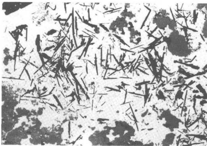
Fig. 38. Sample SO 41-181 FG 8 b. Pyrite (light gray, almost white), containing numerous inclusions of euhedral tabular barite platelets (black) of different size and schalenblende (dark gray) along with small amounts of galena (light gray). In places, the schalenblende also constitutes spheroids (upper right corner of photomicrograph). Polished section, \times 65 .
