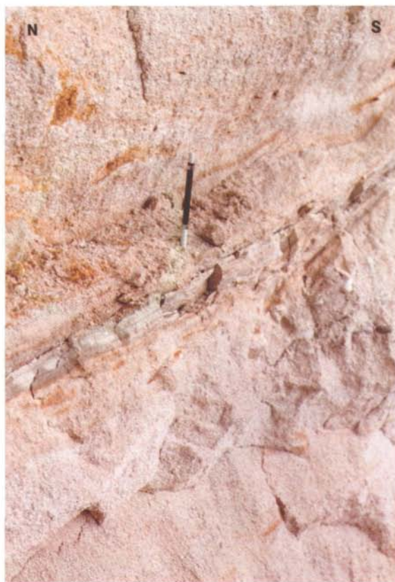
Fig. 72 ▲ Slickenside of the main 120/60 dipping fault. St. Georgen sandpit.
