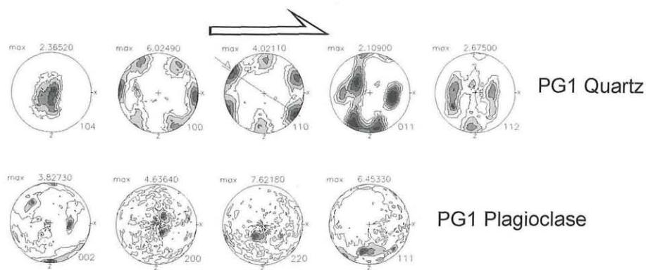
Fig. 4: Quartz LPOs from the Plattengneiss determined by neutron texture goniometry. The (104)-poles have directly been measured and are closely oriented to the c-axes [001]. Stereographic projections, lower hemisphere; logarithmic gradation of isolines; first isoline: uniform distribution; fifth isoline: 85% of maximum.
