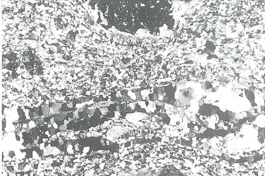
Fig. 3: Representative microfabric from the Plattengneis, with typical quartz layers showing HT microstructures (for explanation see text); crossed polarizers; long axis of photograph about 4mm.
