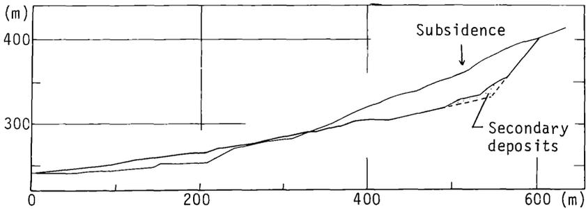
Fig.9 The section of A - A' line before/after the landslide
