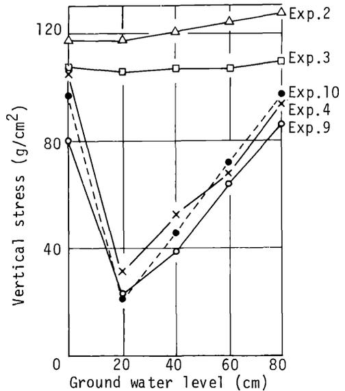
Fig.2 Variation of vertical stress with the ground water level
