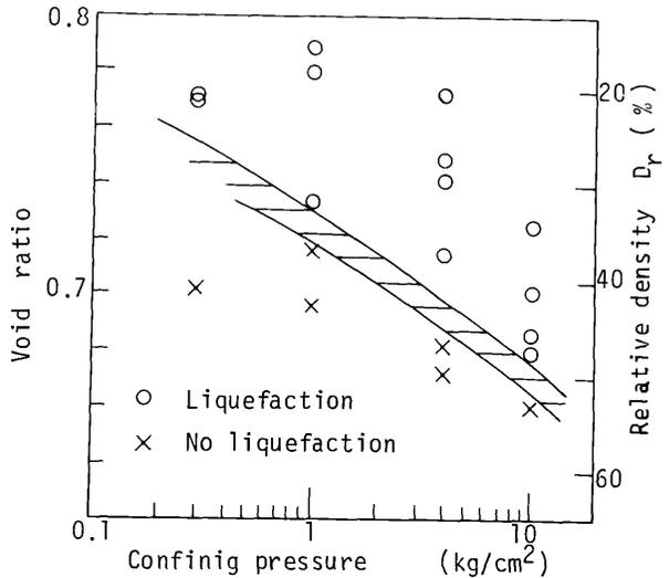
Fig.6 The range of void ratio and confining pressure to cause liquefaction (Reproduced from C. Castro, 1969)
