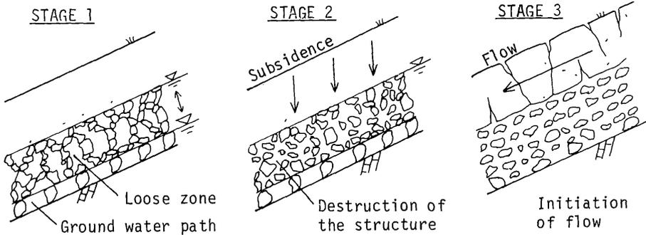
Fig.4 Illustration of the liquefaction caused by subsidence
