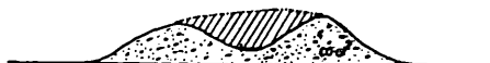
Fig. 1. Box - shaped cross - section of deposits of rapidly moving decelerating debris flow (Aulitzky 1970), observed in the Enterbach / Tirol / Austria
