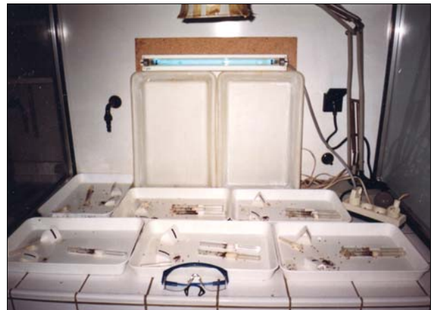
Fig. 2: Experimental device allowing the ants to be conditioned under either only UV light, or only yellow light, or combined UV and yellow light.
