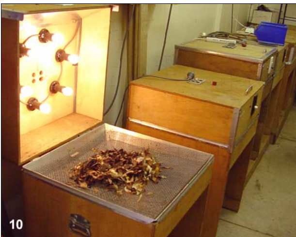
Figs. 8 - 10: Methods used in the fauna surveys at Worsley and Iluka: (8) pitfall traps, (9) suction sampling, and (10) Tullgren funnels.
