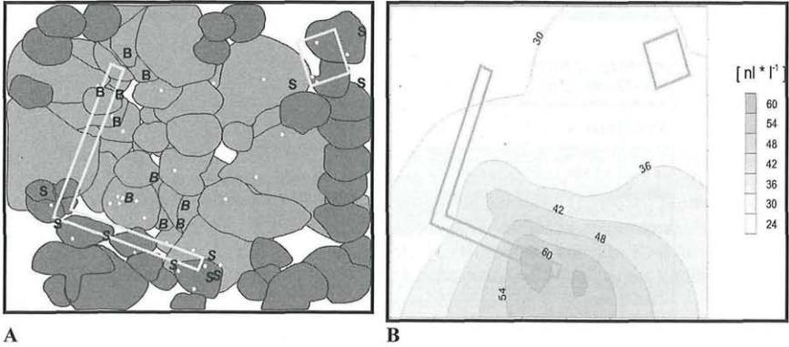
Fig. 6. Experimental site at Kranzberg Forest. A: crown projection of the experimental plot (light-grey = beech; dark-grey = spruce); B: Extension of the experimental  $O_3$  regime in the sun crown as released from the “free-air” fumigation. Frames indicate scaffolding; dots denote the positions of the passive-samplers; B (beech) and S (spruce) indicate the stem positions of the experimental trees.
