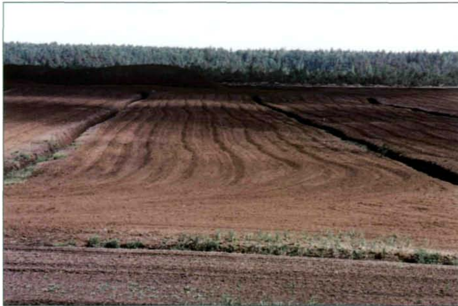
Photo 17: Milled peat excavation area. Sangla bog, Tartumaa district.
