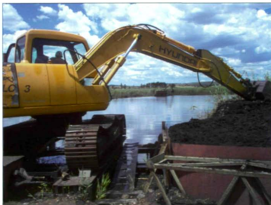
Fig. 5: Peat mining using the floatation peat mining method at Gerhard Minnebron in the Mooiriver Catchment, close to Potchefstroom.
