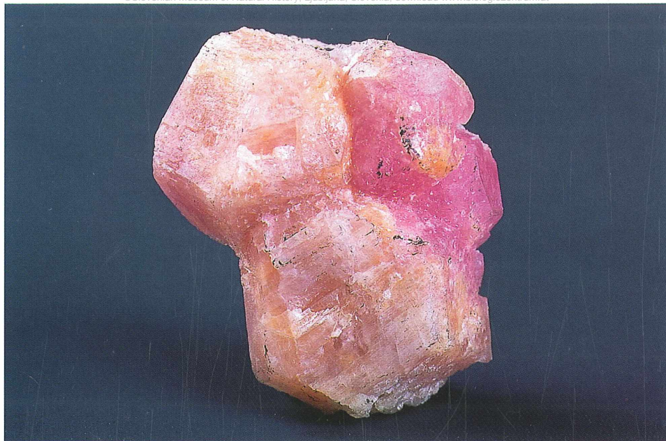
Figure 10: Intergrown corundum and diaspore crystals. Dimensions of the crystals group are 3.2 x 2.0 cm.
