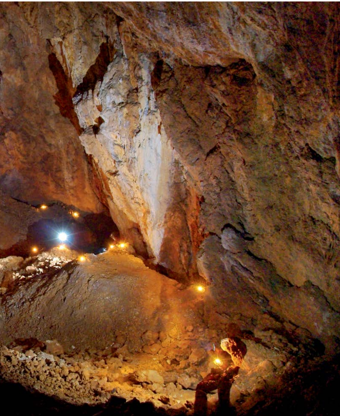
Figure 18. Some karstic ore caves are very large, such as the cave Cok on the Jelovica Plateau: in the partially calcified chamber of the Gothic church size there are, as illustrated by candles, shafts panelled with wooden beams along the walls. The heaps of sand are slagheaps, which is a unique case of slagheaps found below the surface; situation in May 2011.
