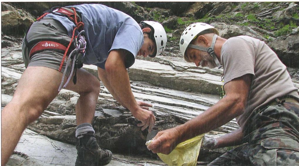
Zaščita s folijo in učvrstitev z mavcem. Protection with foil and stabilisation with plaster.
