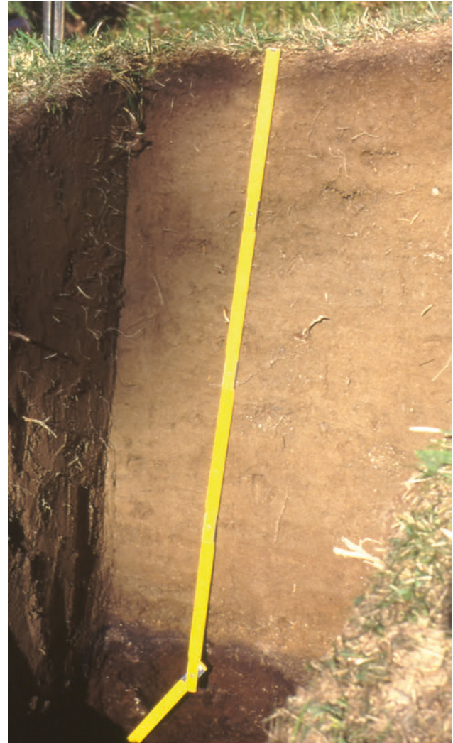
Fig. 7: Soil profile from Horlachtal (Grastalpfeld, 1720 m): the multiple layers of the parent material can be clearly distinguished by the different colours (Geitner 1999: 189) (photograph by C. Geitner 1997).
