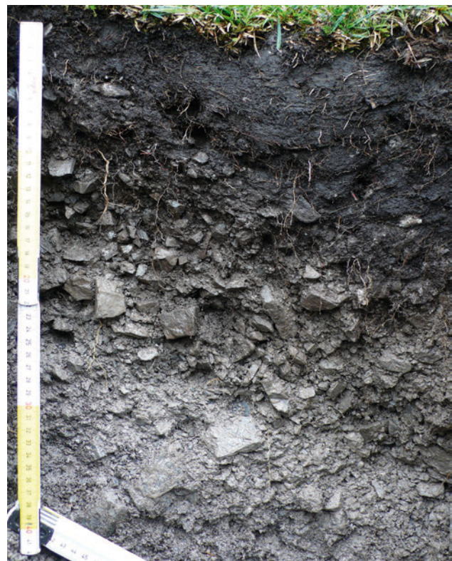
Fig. 3: Soil profile 1 from dolomite debris in Brixenbach valley (1 000 m): the multiple layers of the parent material are clearly identifiable from the varying skeleton content. Photograph by C. Geitner 2008.
