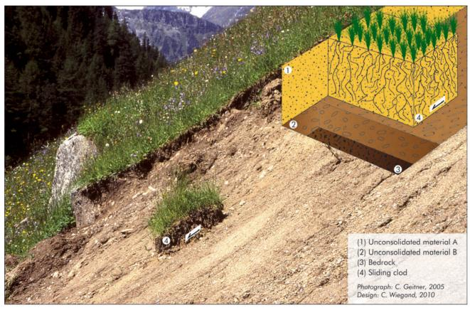
Fig. 3: Schematic diagram and photograph of a shallow landslide near Niederthai, Tyrol.
