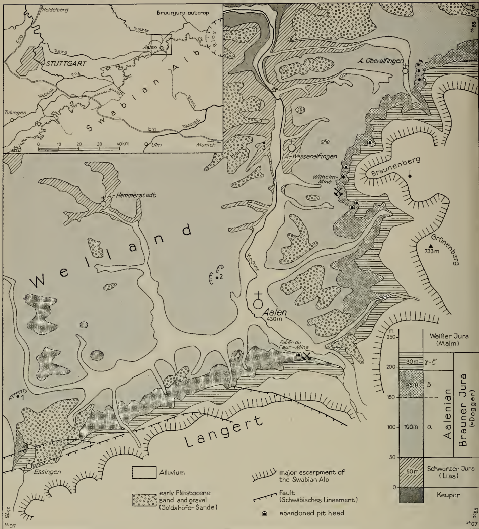
Fig. 1. Geological sketch of the Aalen region with important outcrops in the Aalenian. (1) New brick pit near Essingen (Opalinus-Ton); (2) brick pit in Aalen (Opalinus-Ton); (3) roadside slope in Aalen-Wasseraalfingen "Gewann Hart" (columnar section, fig. 2); (4) brooklet ravine in the Braunjura \beta (WEBER 1964, profile 63); (5) brooklet ravine (columnar section, fig. 3; WEBER 1964, profile 62).
