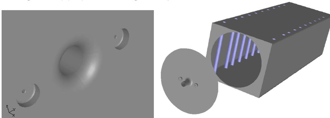
Figure 10 : (a) Injectors of the NFK HRS-DL Burner – (b) Combustion Cell
