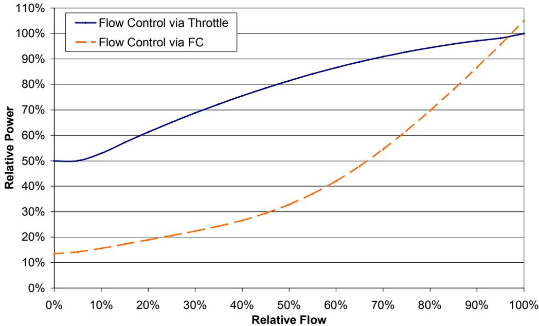
Figure 5: Example for characteristic diagrams of control systems
