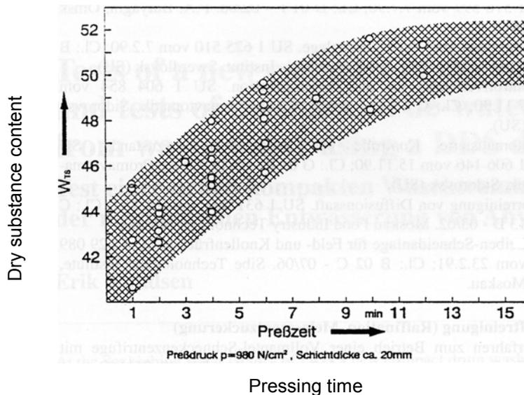
Fig. 10: Capacity of dewatering from the HMP type Regensburg
