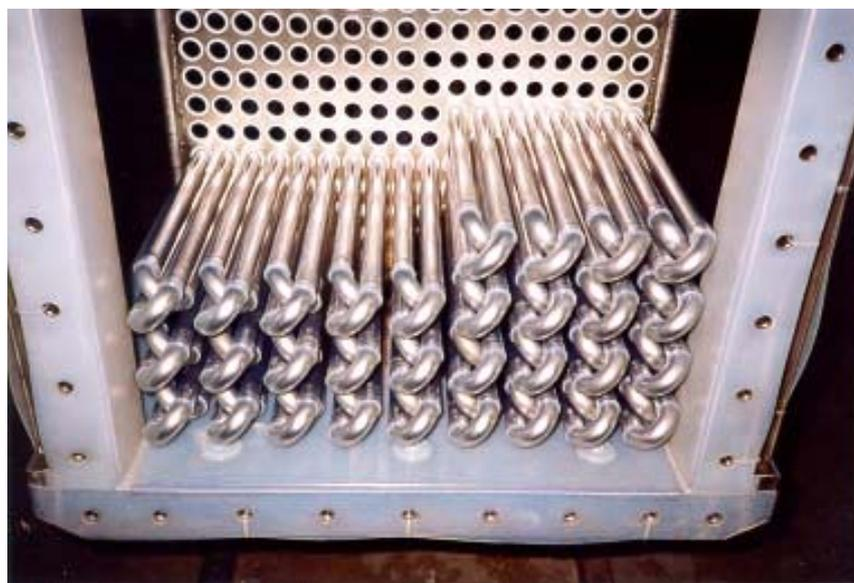
In this case, the required corrosion resistance is achieved by steel tubes enamelled in a two shift procedure with PTFE coating. This multi-layer construction takes especially well into account the different attack qualities of the involved corrosive gas and/or liquid components.
