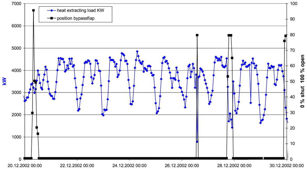
The next data show the performance after elimination of the last lack points in the spring revision 2003. One recognizes acceptable temperature variations and heat extraction loads are above the rated output.
