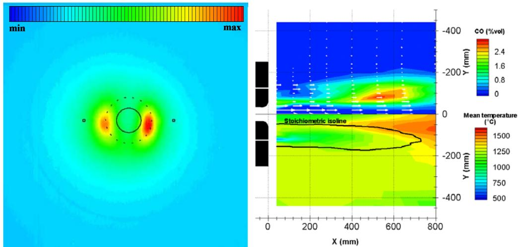
Figure 8 : (a) Chemiluminescence Emission of the OH\* radical – (b) Concentration in CO and mean temperature
