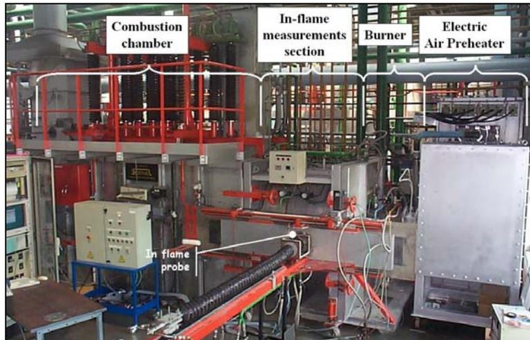
Figure 7 : Test installation at semi-industrial scale
