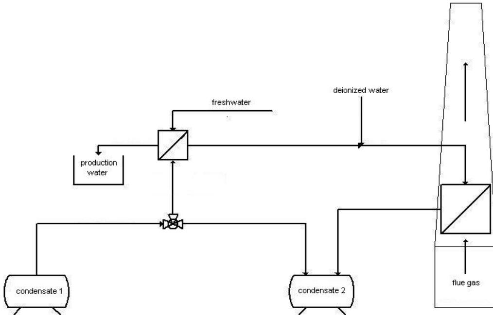
Figure 2: Example for a heat recovery system
