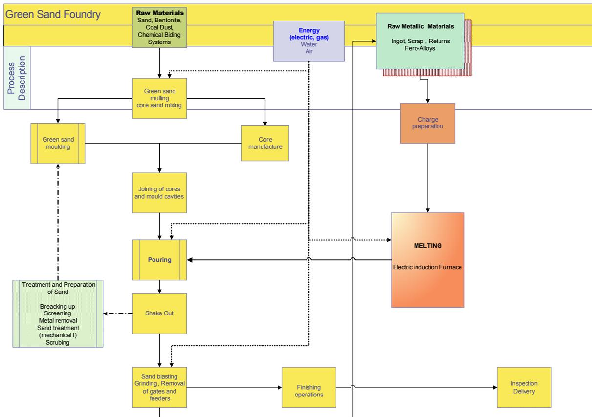
Figure 1: general process flow diagram for PortCast Internet Porto: there are two main flow steams: one for metallic materials that start at the stockyard, go through melting furnaces up to moulding cavities, where the metal take shape during solidification and cooling of molten metal, and another the flow of sand, to make the mould cavities and cores
