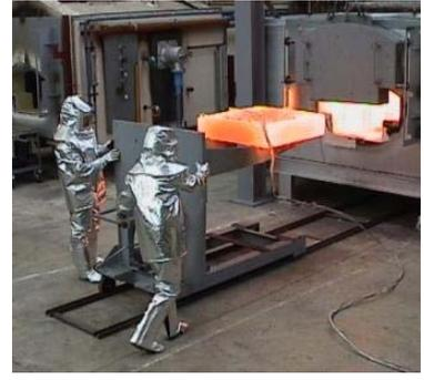
Figure 13 : (a) Loading of the slab, (b) Heating of the slab by the burners, (c) Unloading of the slab
