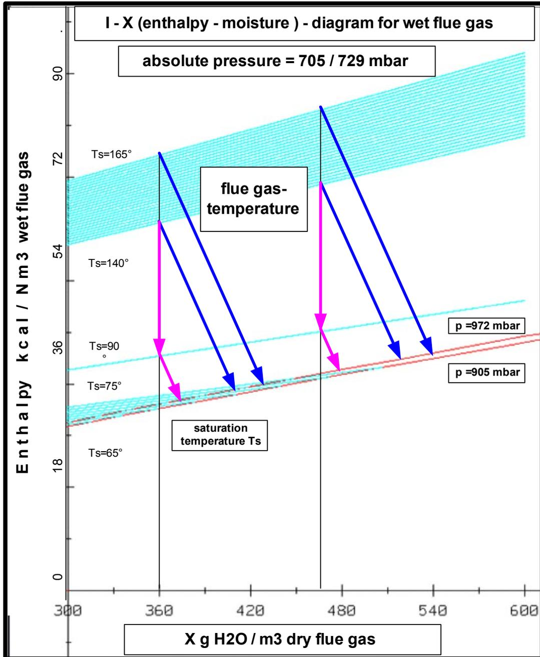
As you can see from the represented data, the effects through the indirect heat extraction are in the same magnitude as they are caused through the changeable operating parameters in normal operation. As a positive effect the drop of the saturation temperature by approximately 2 ° C must be mentioned ( this hypothetical value could also be verified during the test phase by measurement ).
