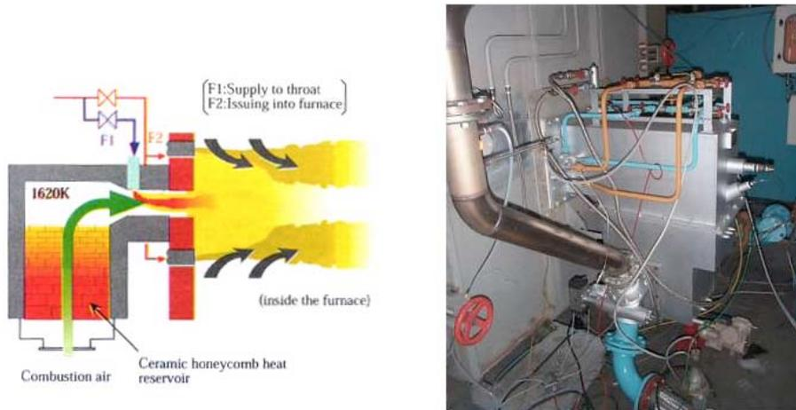
Figure 5 : HRS-DL Burner From the NFK Company (Japan)
