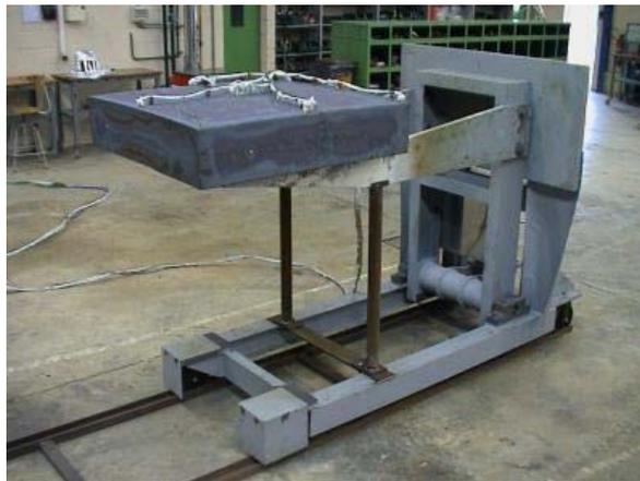
Figure 12 : Instrumented slab on its furnace loader
