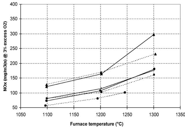
Figure 6 : NOx emissions from burners operating in the flameless oxidation mode, as a function of temperature
