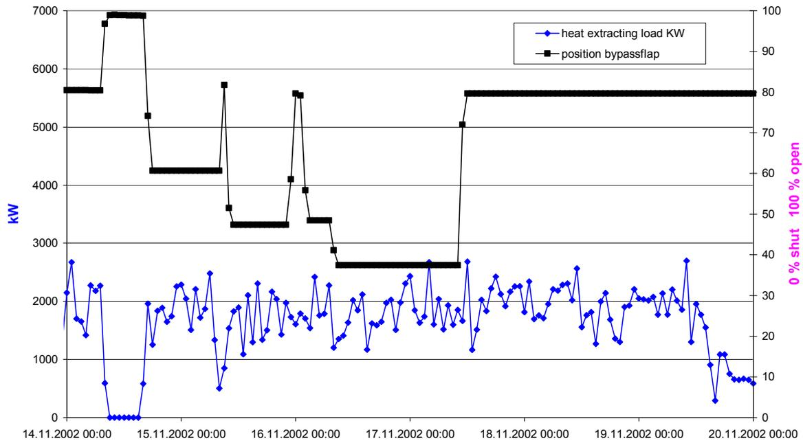
The operating data after implemented optimization. One recognizes that the nominal thermal capacity is already achieved but not yet optimized. Because of irregular cleaning cycles we got temperature rises by pollution of the heat exchanger.
