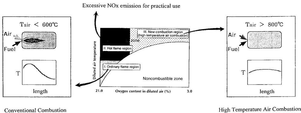
**Figure 4** : Explanation of the lower NO<sub>x</sub> emission level achieved with the flameless combustion mode in comparison with conventional combustion
