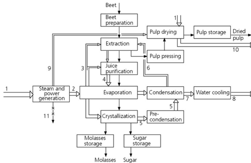
Main energy: 1 Fuel, 2 Steam, 3 Vapours, 4 Hot Juice, 5 Evaporating crystallizer vapour, 6 Hot water, 7 Condenser water, 8 Heat dissipated to the environment, 9 Flue gas to pulp drier, 10 Gas from pulp drier exhaust, 11 Power
