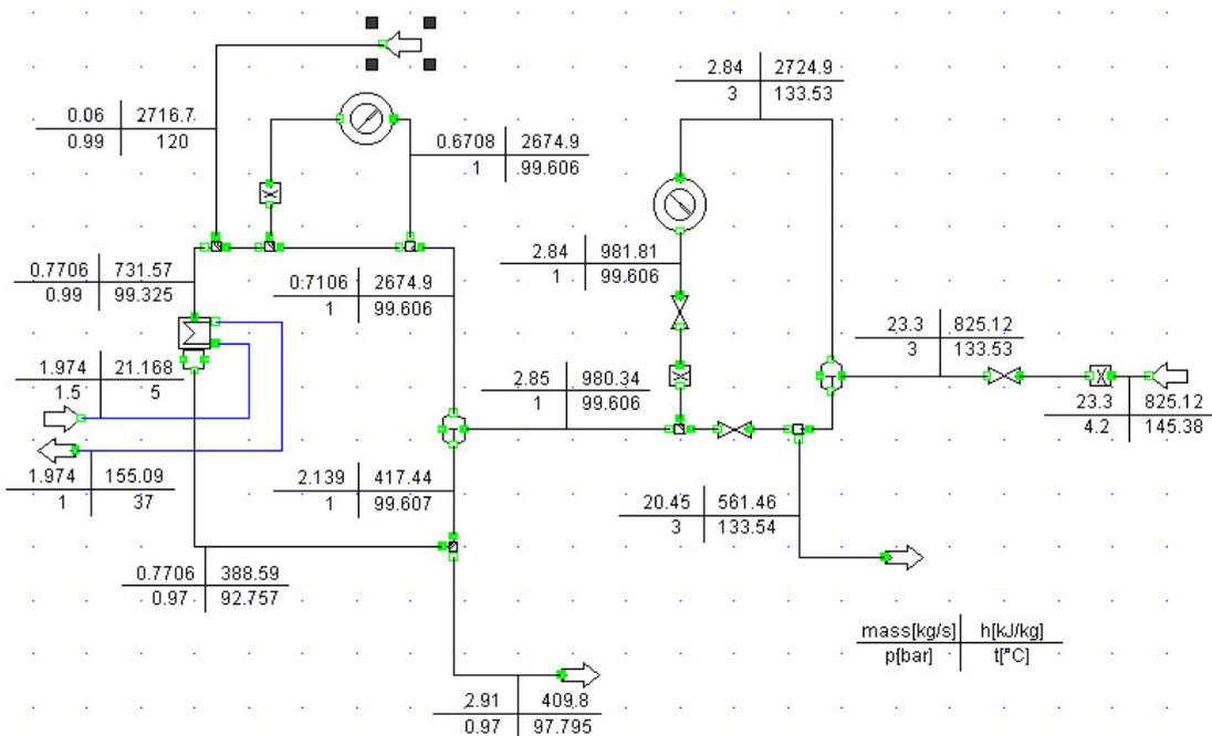
Figure 6: Simulation of taking off condensate
