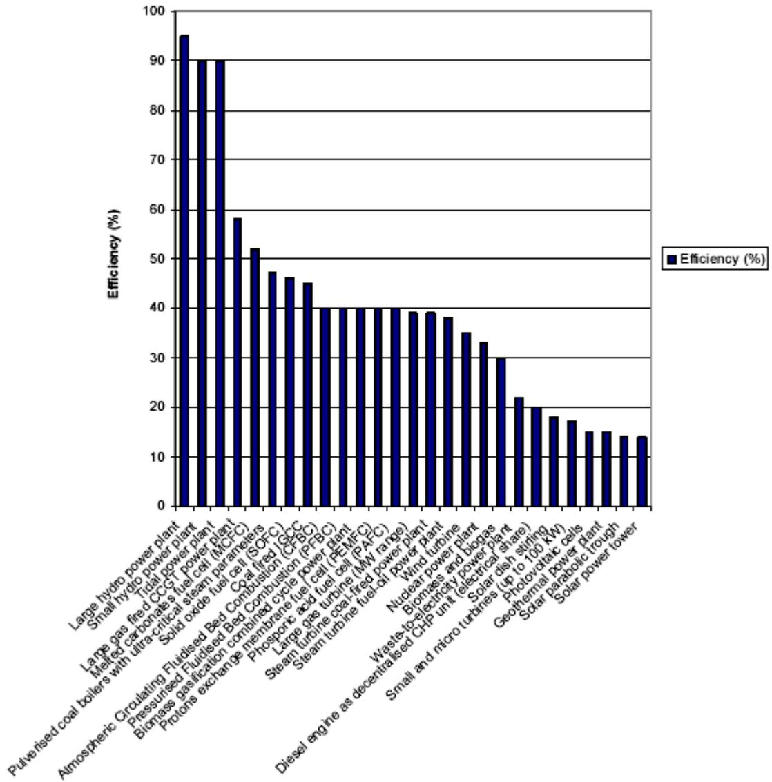
Figure 3.1 Typical energy efficiencies of new generation installations (Eurelectric, 2003)
