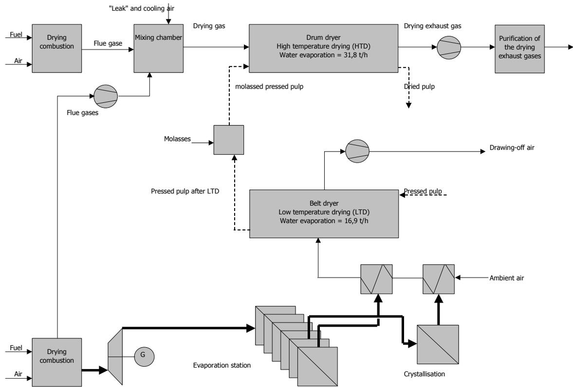
**Figure 17: High temperature drying of beet pulp**
