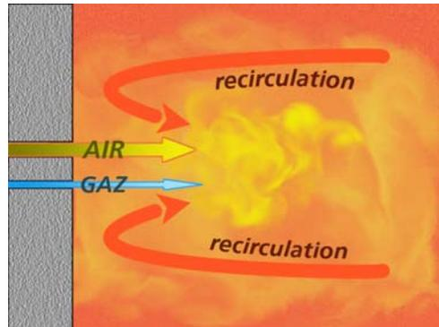
Figure 1 : The principle of flameless oxidation mode
