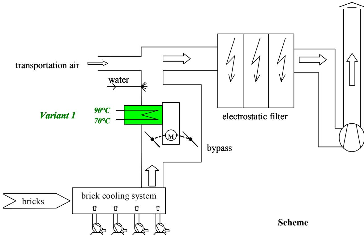
Figure 4: Example for a production heat recovery system
