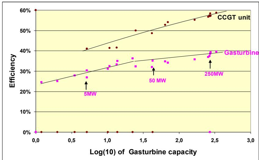
Graph: Efficiency of gas turbines and CCGT units
