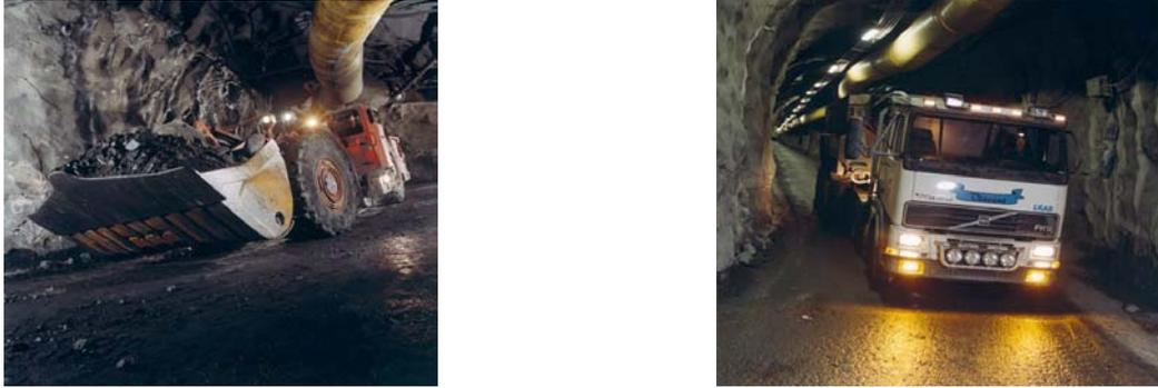
Figure 1. Mine vehicles such as diesel front-loaders and large trucks increase the need for effective ventilation.
