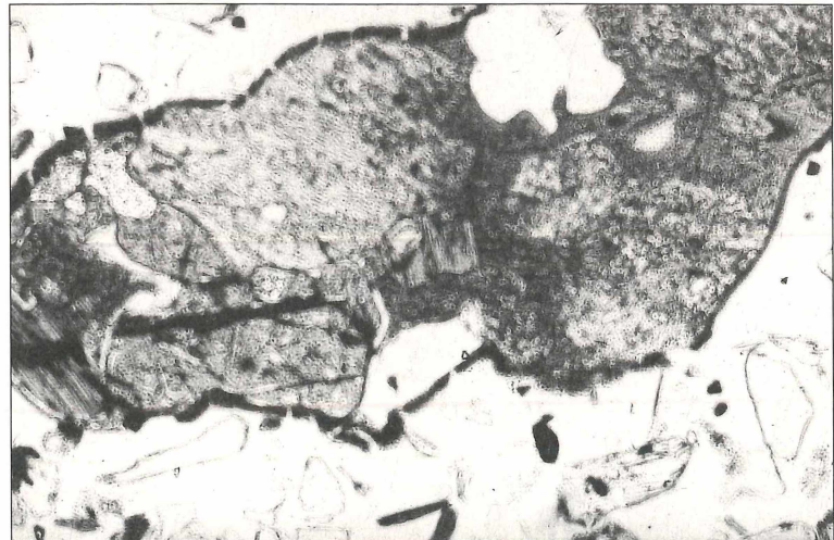
Fig. 4 Micromorphology of the Bh horizon of a sandy Lepti-gelic Podzol (sand grains with black organic coatings); length 3 mm
