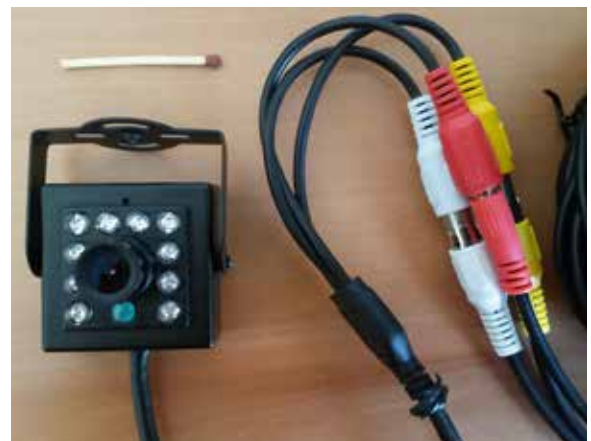
Abb. 2: Benutztes Kamerasystem mit Kamera, Kabel etc., Streichholz zum Größenvergleich. – Camera system with the camera and cables (Handykam.com) used in nestboxes. The compact camera is small and can easily be fitted into nestboxes. It contains a CCD-sensor, adjustable 69° lenses, mono microphone, 10 LEDs emitting infrared (IR) light and can be connected with PCs, monitors and TV by cinch plugs. Image shows a match for size comparison.
