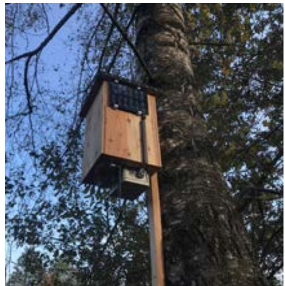
Measuring node on the bottom and solar panel on the back of the nest box.
