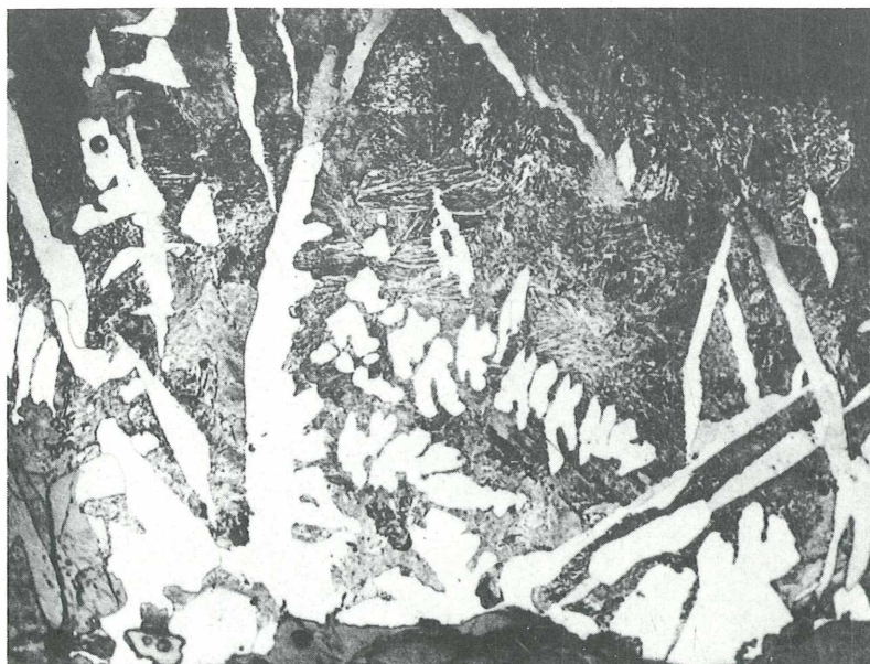
Fig. 6 Unterpullendorf site 1. Structure of the gromp No 3. Metal carbonized to a smaller degree (100 : 1)
