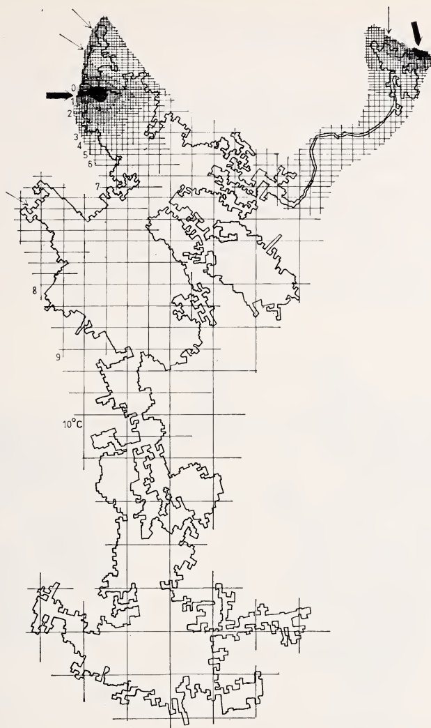
Fig. 3. Distribution of roof air temperature on January 4, 1964. Outside temperature around freezing point ( -0,6^{\circ}\text{C} )
