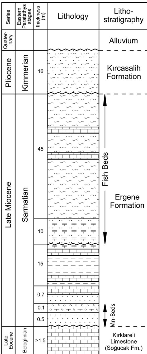
**Textfigure 2:** Pınarhisar, generalized lithological columnar section, adapted from Rückert-Ülkümen et al. (2009: fig. 8).
